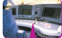
High-Brightness Liquid Crystal Color Display for Railroad Vehicles 1
